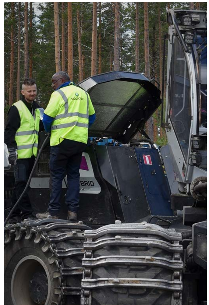
Current R&D is aimed at reducing emissions from forest machines and fuel consumption. Here, hybrid technology is being tested on the Logset 12H harvester.
