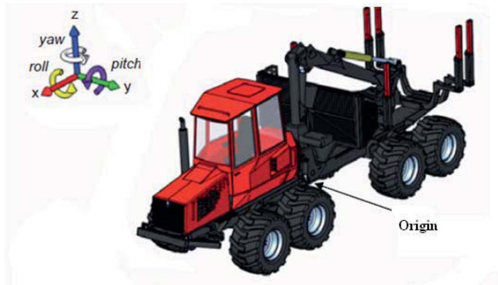
Figure 3.1. Global coordinate system of the forwarder (Olof Karlsson, et al., 2010).
