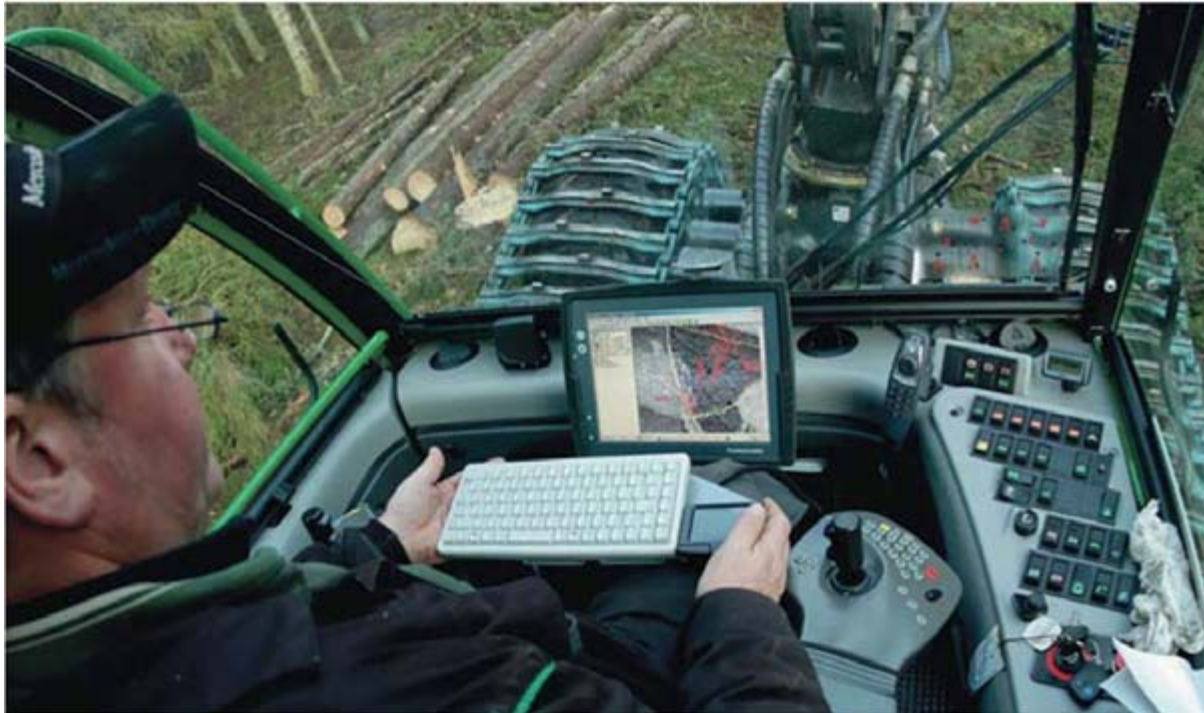
Figure 4. Digital harvester object directives can now be presented on screen in the harvester and forwarder computers according to StanForD-standardisation. This enhance traceability at the pile level and is a tool for atomised communication as harvester production reports linked to forwarding operations and reports.
