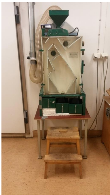
Figure A1-3. Gravity separator. The apparatus where the seeds were separated from the wing fragments and the filled seeds were separated from the non-viral seeds.
