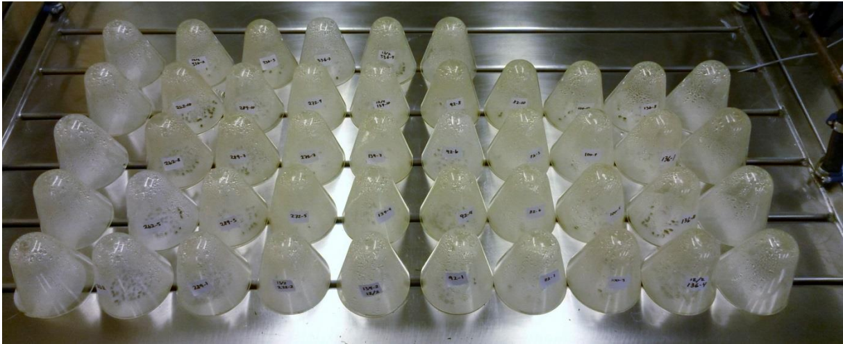
Fig A1-4. Jacobsen's apparatus. The seeds were put on filter papers on a germination table under translucent plastic cups in order to germinate. Here the conditions were 16h at 20°C and 8h at 30°C with a constant light exposure.
