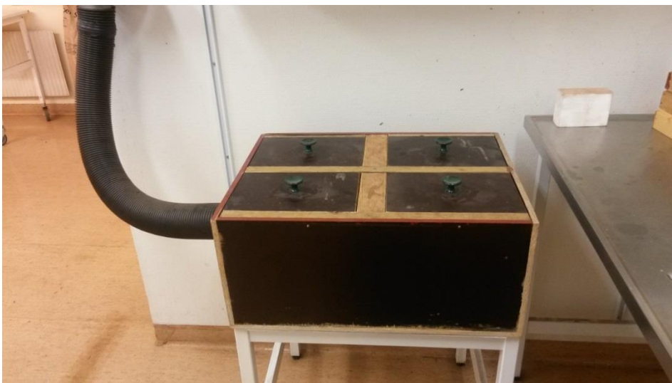
Figure A1-2. Drying equipment. The seed material was dried by the use of the ventilation system.
