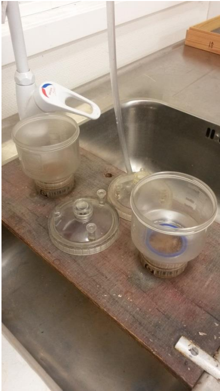
Figure A1-1. Soaking apparatus. The apparatus where the seed material was soaked with water in order to make the wing detach from the seed.
