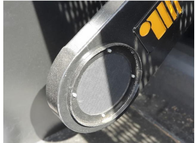
Probe for measurement of moisture content in wood chips.
